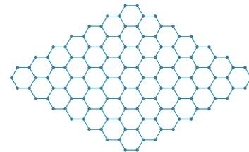
Fig. 5: Structure of a graphene layer.
