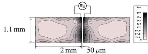
Fig. 2: Top view and current distribution of a two patch antenna, operating at 66 GHz.
