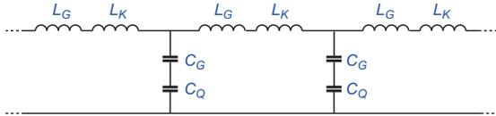
Fig. 4: Equivalent circuit model of a CNT over metallic ground plane.
