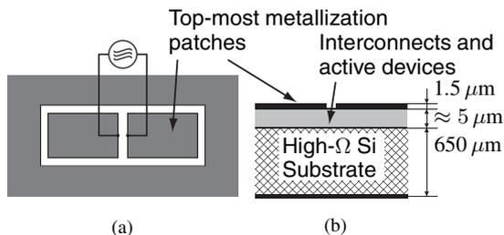
Fig. 1: A top view (a) and a cross-section view (b) of a chip with an integrated antenna.
