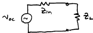
where  $Z_{in}$  is the input impedance of the antenna as a transmitter,
