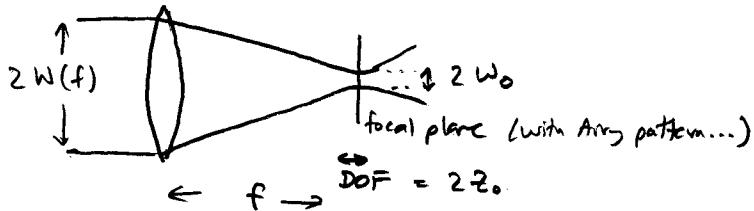
We can estimate the DOF by modelling the wave as a Gaussian beam. If we put  $z=0$  at the focal plane,
